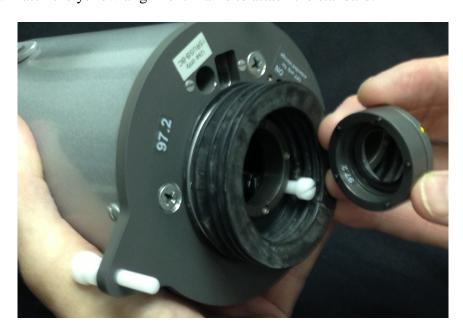
4. Calibrate the instrument. Adjust the reading with the gain knob to match the reflectance value for the standard. The reflectance value is found on the standard and on the base of the instrument. After
