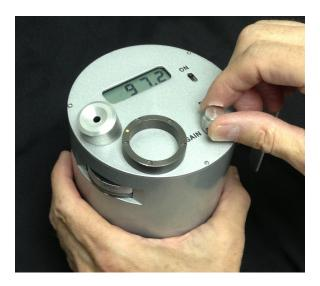
5. Adjust the center support leg to compensate for the mirror thickness. For a first surface mirror adjust the support to the fully counterclockwise position. For a second surface mirror start at the fully counterclockwise position and adjust the support by 1 full turn in the clockwise direction for each 0.05 inches thickness.
