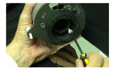
6. Place the 15R on the test sample. Adjust the outer legs to locate the reflected image within the aperture by watching for a reading on the display.
